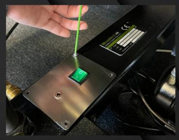
push wiring through tube
